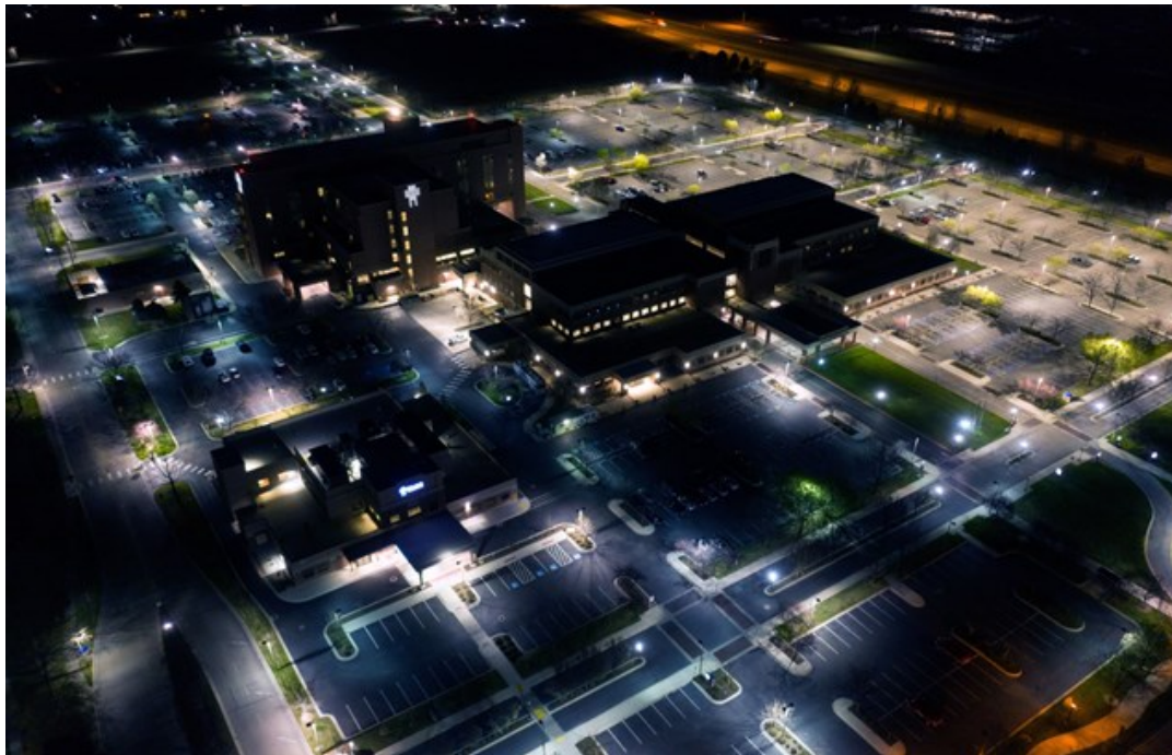
Figure 1. Parking lots on the left side of the property are lit using traditional metal-halide lighting and parking lots on the right side are lit using LEDs. Notice the difference in uniformity levels.
